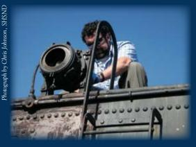
As part of the restoration project of the Northern Pacific Locomotive 2164 at Camp Hancock State Historic Site, Bryan Turnbow, SHSND preparator, is shown here removing the lens from the rear light of the locomotive's tender, or coal car, prior to its repainting. Right, a contractor with Indigo Signworks of Bismarck applies new lettering to the freshly-painted tender.
